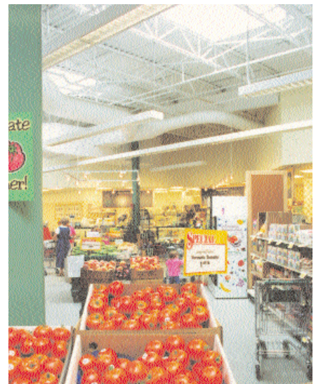
In this grocery store, skylighting provides high illumination, superior lighting quality, and net energy savings
