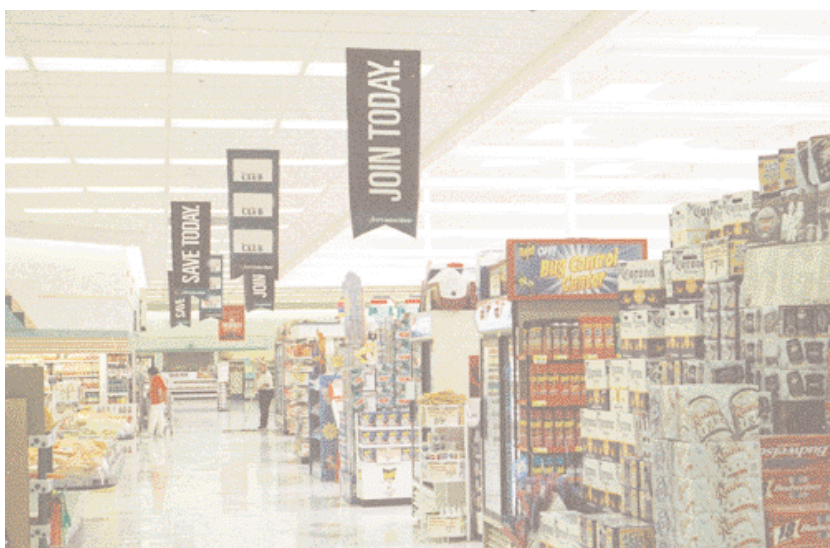
A raised ceiling pulls customers into the skylit center of this grocery. A conventional dropped ceiling rings the perimeter.
