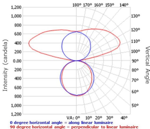
**Figure 6:** Example of a Polar Plot, Candela Distribution
