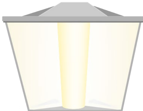
Figure 3: Isometric view of a troffer with a luminous basket and luminous panels on each side. The luminous shape would be represented by a 2D luminous rectangle because a complex shape is not permissible in LM-63.
