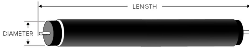
Figure 1: Dimensions of linear replacement lamps to be reported on the application form.
